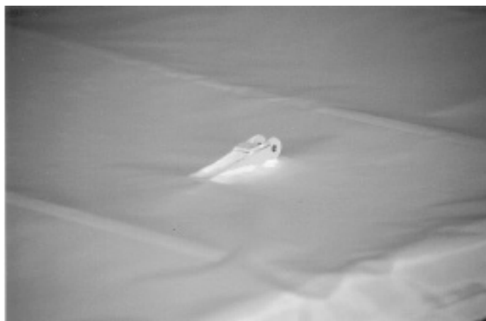
Figure B-2 Fabric Cut to Allow Lift Strut Bracket Ears to Protrude
