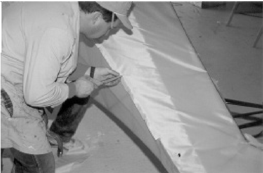
Figure D-5 Trimming Fabric for Proper Overlap Along Longerons
