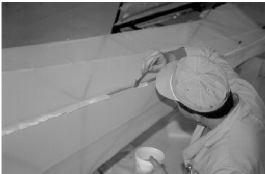
Figure D-7 Bonding Side Fabric Overlap to Belly
