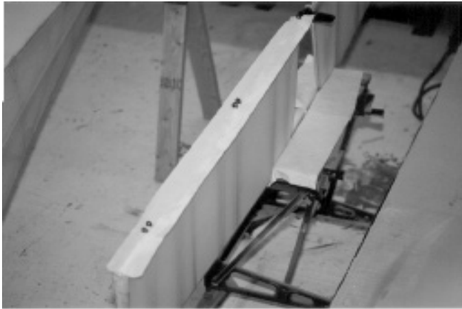
Figure I-11 Elevator Leading Edge Finishing Tape
