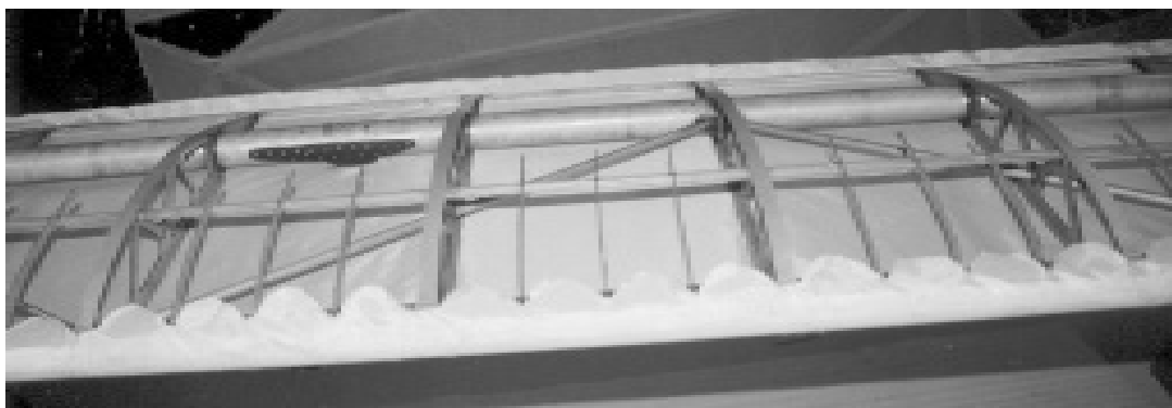
Figure B-1 Leading Edge Overlap with Scallops to Clear Ribs
