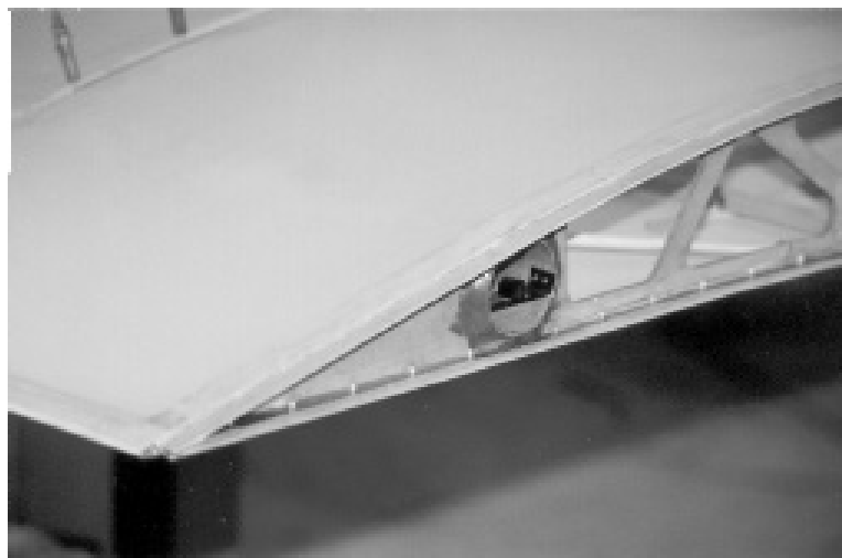
Figure B-6 Wingtip Mounting Strips Riveted to Rib #10 Capstrip
