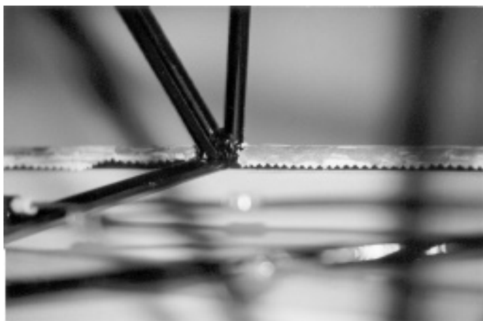
Figure C-7 Completed Fabric-to-Structure Bond
