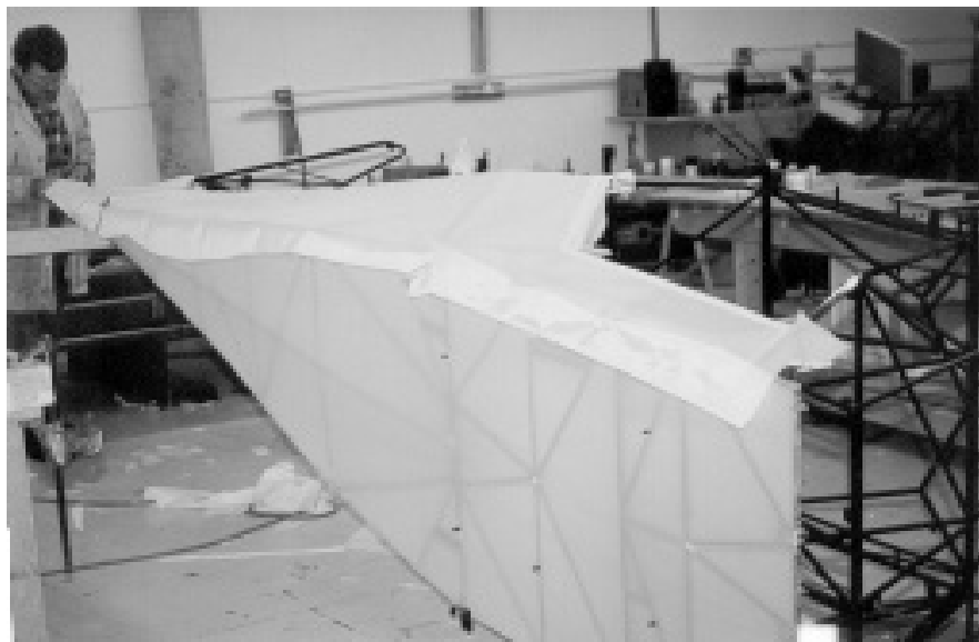
Figure D-1 Fabric Rolled Out and Trimmed on Side of Fuselage
