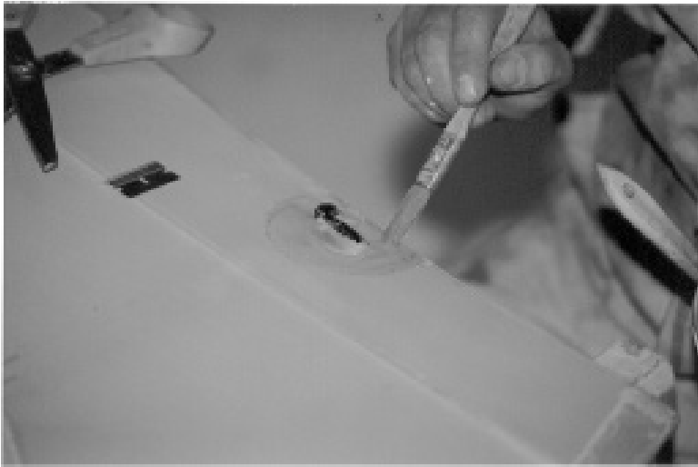
Figure I-6 Horizontal Stabilizer Strut Doily
