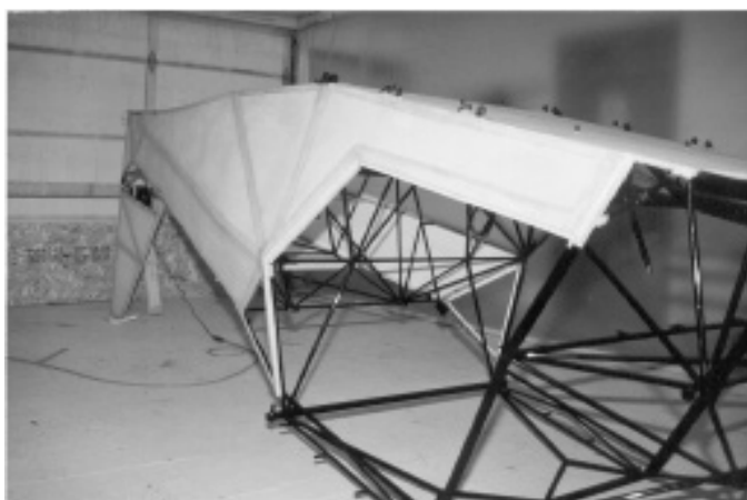
Figure I-3 Fuselage Side Finishing Tapes
